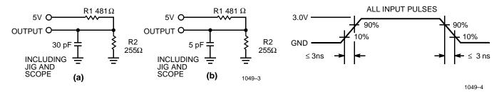
Equivalent to: THÉVENIN EQUIVALENT OUTPUT O  $\frac{167\Omega}{W}$  O 1.73V
