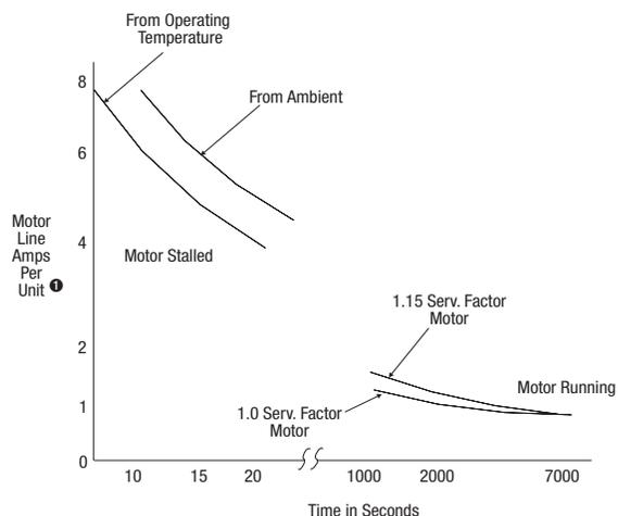
Motor protection, either inherent or in the motor control, should be selected to limit the stall time of the motor.
