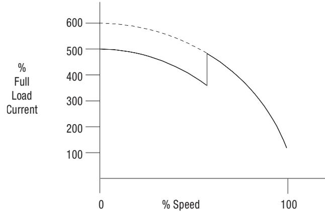
The motor speed can determine the amount of current surge that occurs at transition. Transfer from reduced voltage to full voltage should occur at as close to full speed as possible. This also minimizes the amount of surge on the line.
