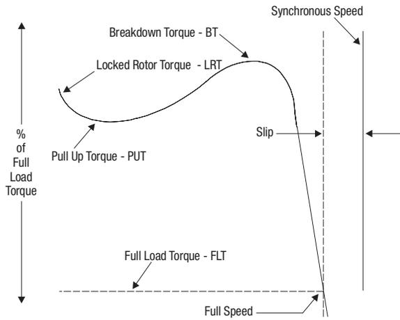
**Locked-Rotor Torque (LRT)**
