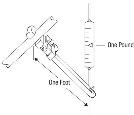
Torque is merely a turning effort. In the previous illustration, it takes one pound at the end of the one foot wrench to turn the shaft at a steady rate. Therefore, the torque required is one pound  $\times$  one foot, or one ft-lb. If the wrench were turned twice as fast, the torque required would remain the same, provided it is turned at a steady rate.
