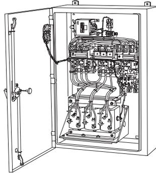
All forms of reduced voltage starting affect the motor current and torque characteristics. When a reduced voltage is applied to a motor at rest, the current drawn by the motor is reduced. In addition, the torque produced by the motor is a factor of approximately the square of the percentage of voltage applied.
