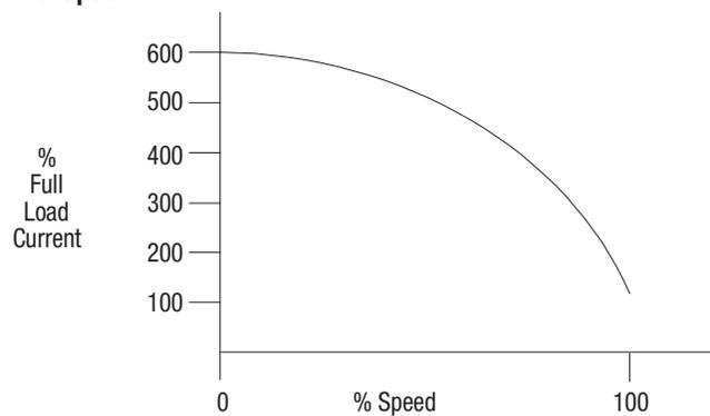
In addition to high starting currents, the motor also produces starting torques that are higher than full load torque. The magnitude of the starting torque depends on the motor design. NEMA publishes standards for torques and currents for motor manufacturers to follow. Typically, a NEMA Design B motor will have a locked rotor or starting torque in the area of 180% of full load torque.
