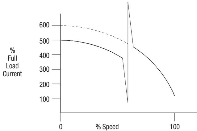
**Figure 6.4 Closed Circuit Transition**
