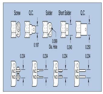
Standard Parallel QC used on -00B and -00E (0.205 x 0.032) Standard Parallel QC used on -00R and -00T (0.187 x 0.020) Vertical Twist QC used on -50B and -50E (0.205 x 0.032) Vertical Twist QC used on -50R and -50T (0.187 x 0.020) Vertical Straight QC used on -60B and -60E (0.205 x 0.032) Vertical Straight QC used on -60R and -60T (0.187 x 0.020)
