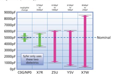
It is clear that the capacitance can change as a result of an increase (or decrease) in temperature, applied voltage and as a result of ageing. If the capacitance has reduced, so too will the insertion loss performance.
