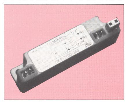
SKPC100 is one of the new generation of Semikron Power Control Modules (SEMI-PCM). The new design allows triggering of a wide range of SCR's for both zero voltage or instantaneous switching applications. Thus forming the basis of very high power solid state relays. The SKPC100 is particularly suitable for highly inductive or large in-rush current type loads.
