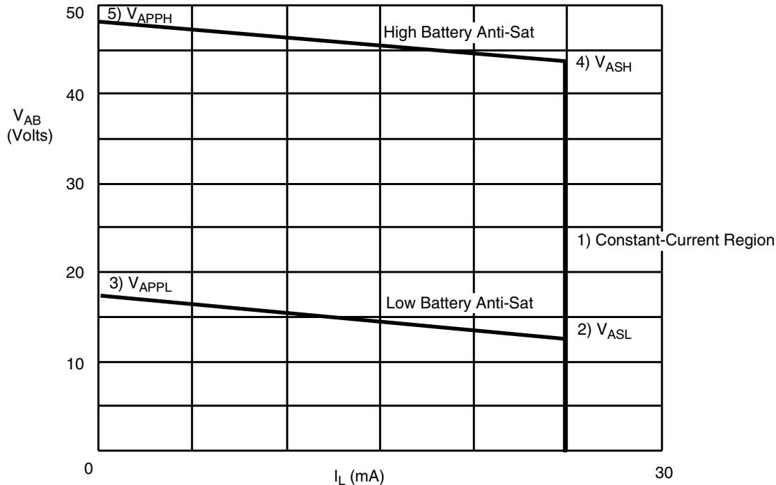
**Figure 1. Typical  $V_{AB}$  vs.  $I_L$  DC Feed Characteristics**
