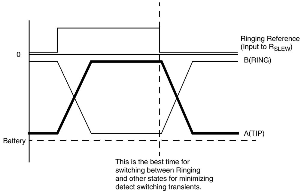
**Figure 2. Ringing Waveforms**
