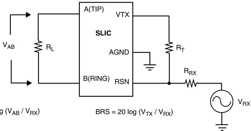
$$I_{L4-2} = 20 \log (V_{AB} / V_{RX})$$
