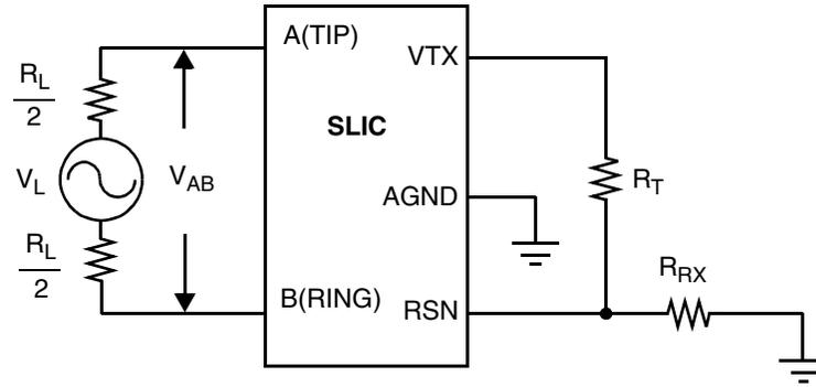
$$I_{L2-4} = 20 \log (V_{TX} / V_{AB})$$
