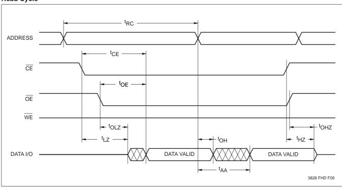
Note: (3)  $t_{LZ}$  min.,  $t_{HZ}$ ,  $t_{OLZ}$  min., and  $t_{OHZ}$  are periodically sampled and not 100% tested.  $t_{HZ}$  max. and  $t_{OHZ}$  max. are measured, with  $C_L = 5pF$ , from the point when  $\overline{CE}$  or  $\overline{OE}$  return HIGH (whichever occurs first) to the time when the outptus are no longer driven.
