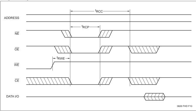
Note: (5) The Recall Pulse Width  $(t_{RCP})$  is a minimum time that  $\overline{NE}$ ,  $\overline{OE}$  and  $\overline{CE}$  must be LOW simultaneously to insure data integrity,  $\overline{NE}$  and  $\overline{CE}$ .
